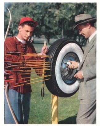
was checked before these twenty arrows pierced the tube, checked after the arrows were removed. There was no loss of air pressure!
