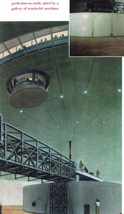
Navy centrifuge at Johnsville, Pa., one of several in use to simulate acceleration force
